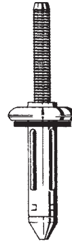
FIGURE 6.7 Fasteners used by one manufacturer to attach through-fastened roofing to purlins and to one another. (The scrubolt is used only for attachment to purlins.) (Butler Manufacturing Co.)
